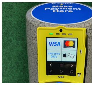
Use the supplied 13.56mhz VendaCard to test the VendaVolt Cashless Nayax Payment and Charger 32A output of 220~240 volts AC. The handshake with the server is only a few seconds and then the count up on the 2x16 LCD will indicate the Nayax portion if functioning for the cashless payment. The VendaVolt Clear Token Cellular Phone App instructions are the customers cell phone.
