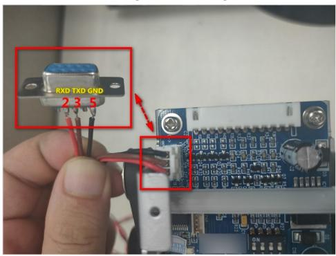
1.2 Wiring method of card dispenser (USB to 232 converter)
