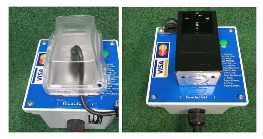
2. Plug in the power cord of the washer or dryer into the VendaVolt Outlet. Secure the power cord plug with the rubber protected "U" clamp and security screw. Last step is to plug in the VendaVolt power cord plug into the mating outlet source for 110~120V or 220~240V. Use a "Loctite" adhesive on the metal pins of the plug to ensure the plug can not be removed from the outlet without management authorization.
